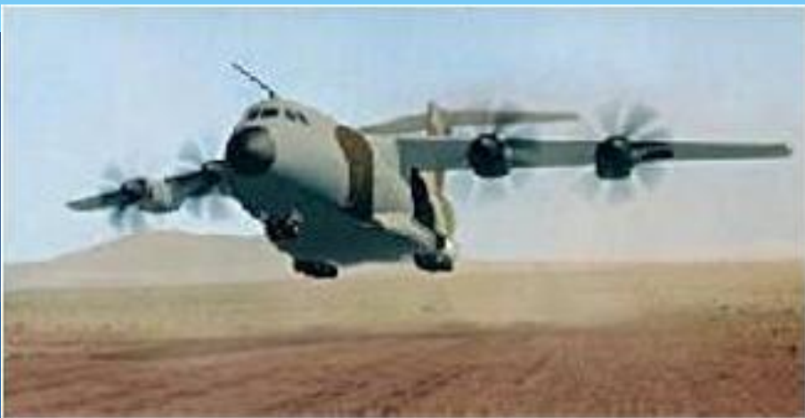
Military Transport Aircraft Wingspan : 42,4 m Length: 42,2 m Powerplant : TP400 AeroProp 11.000 SHP
